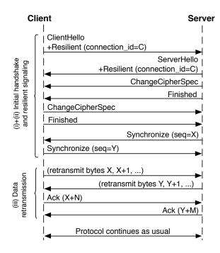
Figure 2: Reconnection procedure in TLS.
