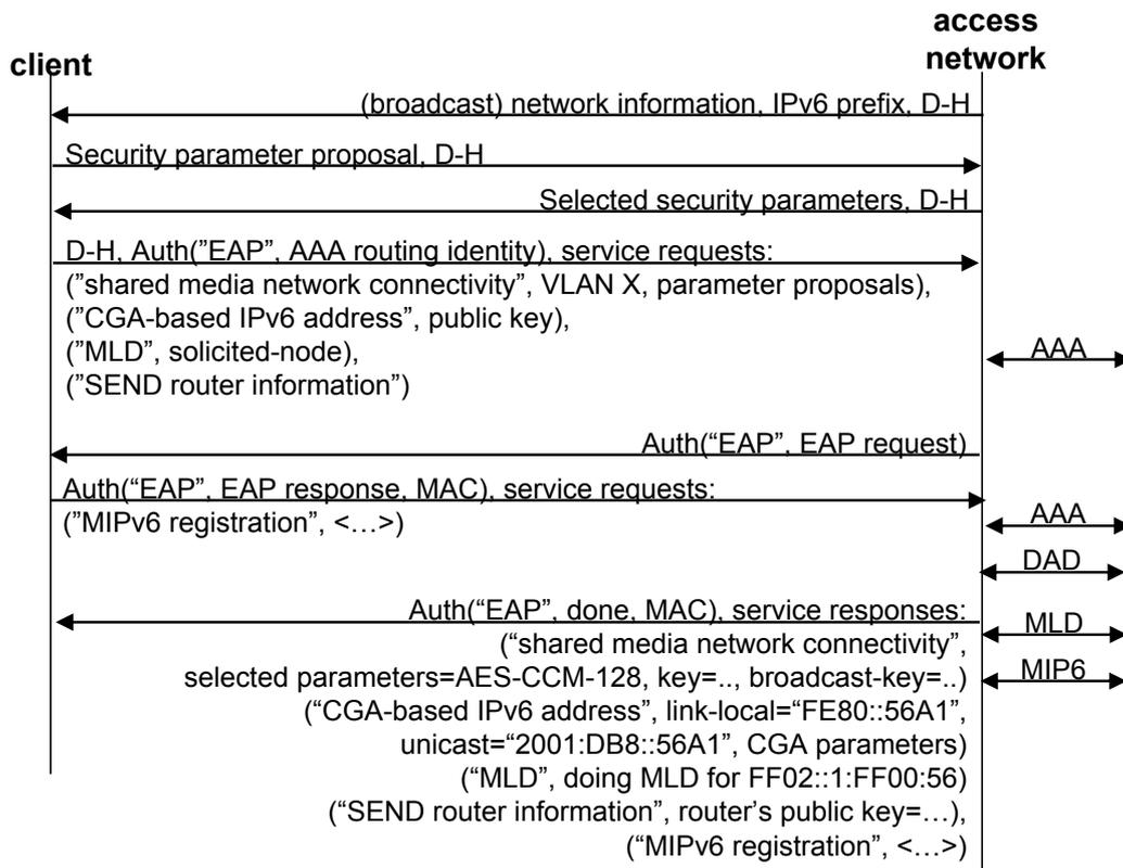
Fig. 2. NAP and IPv6 network attachment.
