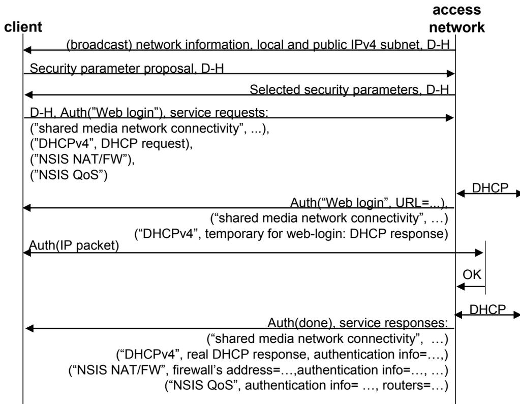
Fig. 3. NAP with IPv4 network attachment.
