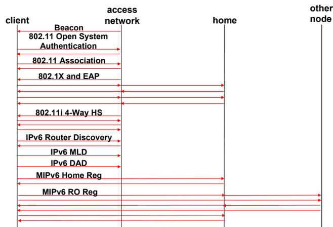
Fig. 1. IPv6 network attachment with existing protocols.
