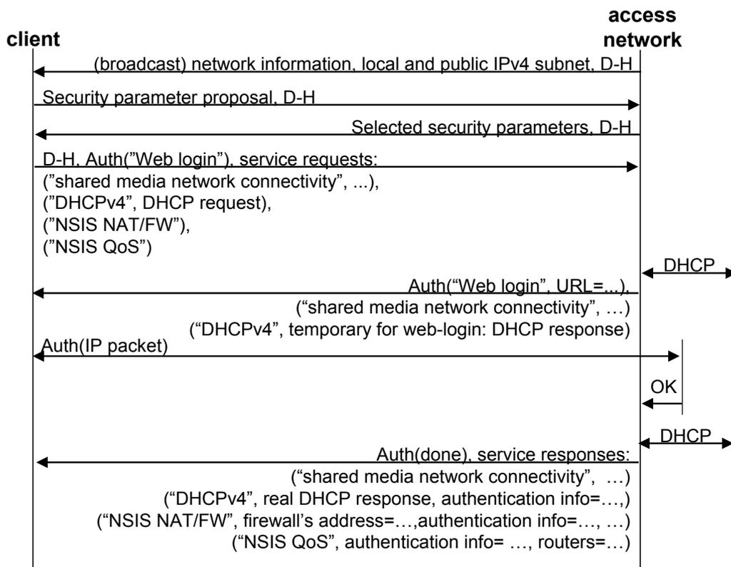
Fig. 3. NAP with IPv4 network attachment.
