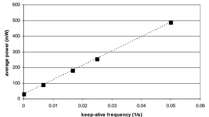
Fig. 3: Average 3G power consumption of keep-alive messages (with acknowledgment) with different intervals. The least-squares fitted line corresponds to 9200 mJ/keep-alive plus 29mW background consumption.
