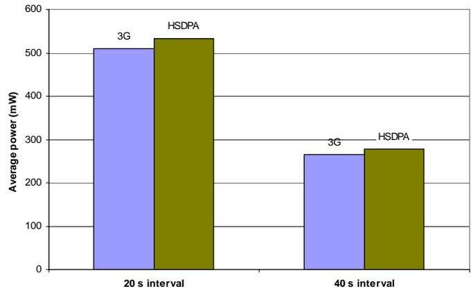
Fig. 5: Average power consumption of a keep-alive exchange (with acknowledgment) on Nokia N95, comparing 3G (without HSDPA) with HSDPA.
