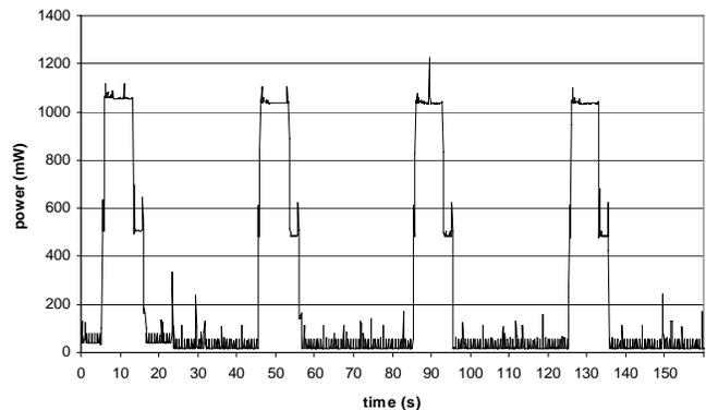
Fig. 1: Power consumption trace of keep-alive messages (with acknowledgment) in 3G with 40-second interval.
