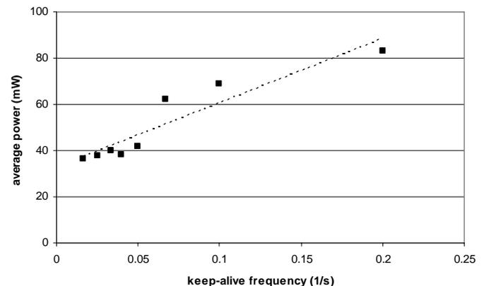
Fig. 6: Average Wireless LAN power consumption of keep-alive messages (with acknowledgment) with different intervals. The least-squares fitted line corresponds to 280 mJ/keep-alive plus 33 mW background consumption.
