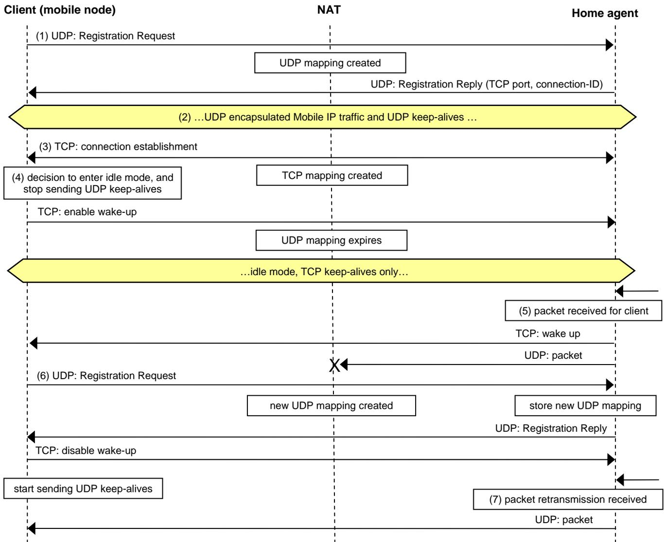
Fig. 7: Overview of TCP Wake-Up with Mobile IPv4.
