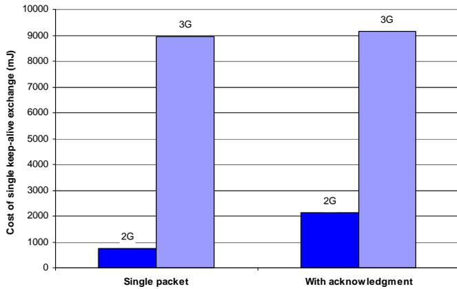
Fig. 4: Energy consumed by a single keep-alive exchange, for both 2G and 3G, with and without acknowledgment packet.
